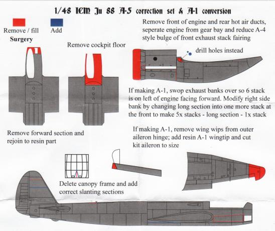
Delete upper panel line on vertical stabilizer, delete control cable panel from right side cockpit. If making A-1 reduce rear of dinghy hatch by 10mm and also delete hand holds along top of fuel cell on the left side. Add missing outer bomb bay hinge line to both sides.
